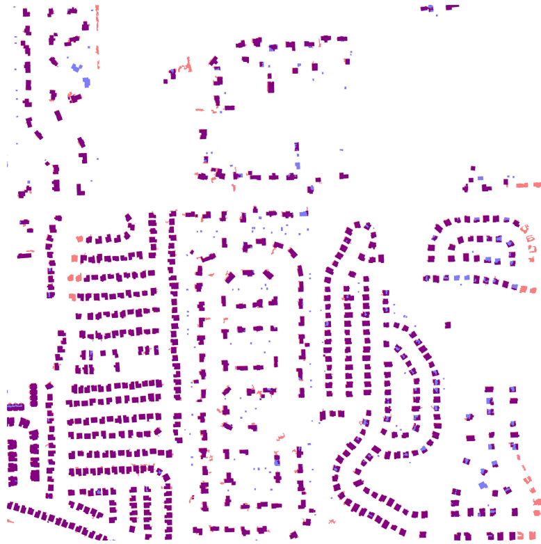
(a) Classification of the tile in Figure 5.2a using a model trained on the tile in Figure 5.1b. Red areas are false positive areas, blue areas are false negatives, and purple areas are true positives.
